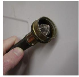
2. Check all hoses for visible signs of deterioration including cracks, blisters, corrosion or material wear.
