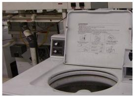
2. Wipe the machine's top, front and side panels clean as needed. If detergent, bleach or other washing products are spilled on the cabinet, wipe immediately. Some products will cause permanent damage if spilled on cabinet. Thoroughly rinse and dry all surfaces after cleaning them.
